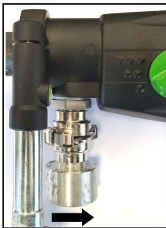
Dust which occurs during your work is hazardous to health. That is why it is advisable to use a deduster and to wear a dust mask on dry drilling. Place the adapter for the dedusting unit onto the tool's connector and turn into the direction of the arrow up to the stop. As a suitable wet/dry deduster, our DSS 35 M iP is available as add-on. The use of a dedusting system is also a prerequisite for optimal cutting performance of the bit (air cooling).
