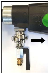
Place the adapter with the ball valve onto the tool's connector and turn into the direction of the arrow up to the stop. Connect the tool to the water supply system or a water pressure vessel using the push fit nipple.
