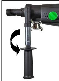
For manual drilling, the **PLD 182.1 NT** may be used only together with its additional handle which comes with the tools.
