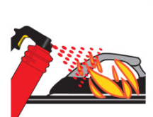
... for use on electrical appliances up to 1000 V, min. spray distance 1 m
