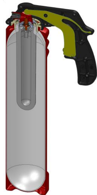
3D Sectional view with unfilled and filled force element (coloured grey)
