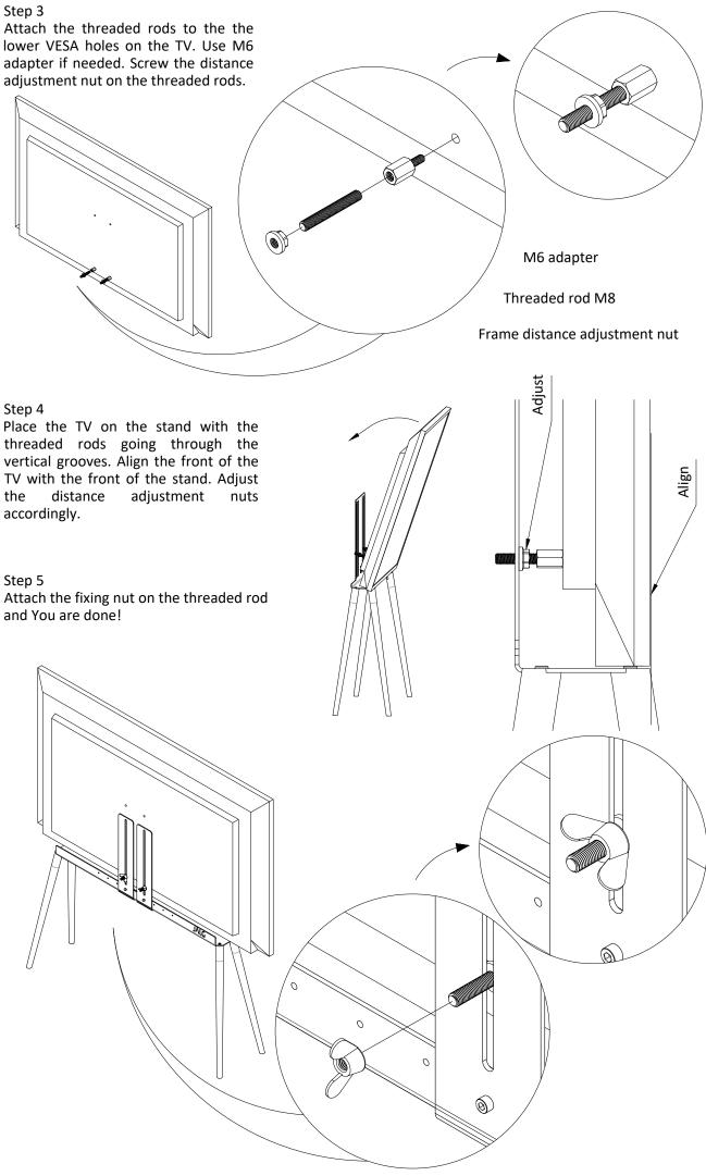
threaded rods going through the vertical grooves. Align the front of the TV with the front of the stand. Adjust the distance adjustment nuts
